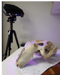
Solutionix C500 Structured Light Surface Scanner at Archaeology Laboratories, the University of Queensland
